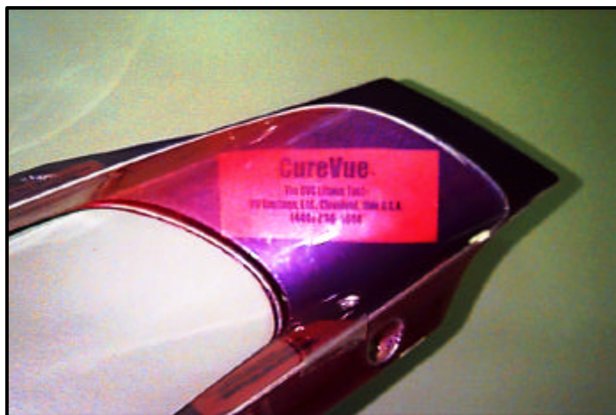
Fig. 2. After UV exposure the 3dr indicates UV distribution over the surface. Note the effect UV blocking film had on the 3DR indicator underneath.
