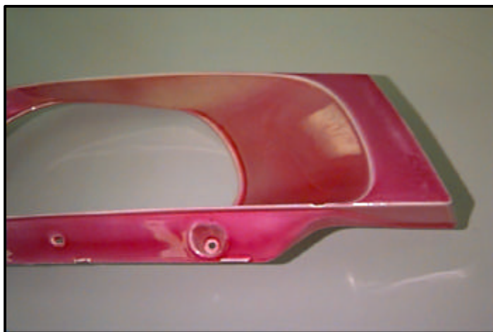
Fig. 1. Before: A thermoplastic automotive 3DR before UV exposure.
