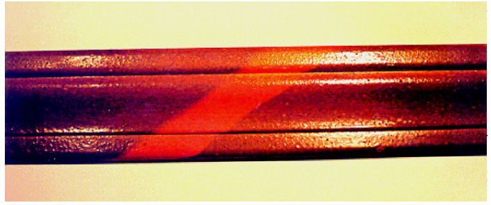
Fig. 5. Above: The 3DR indicated not only a contour irradiance issue but also a UV shadow issue for this part. Note the areas that vary directly with the contour. This indicates the top lamp on this flat line operation was not operating properly – perhaps the part was run before the lamp reached full operating intensity. Additionally, some foreign object cast a shadow on this part during cure.
