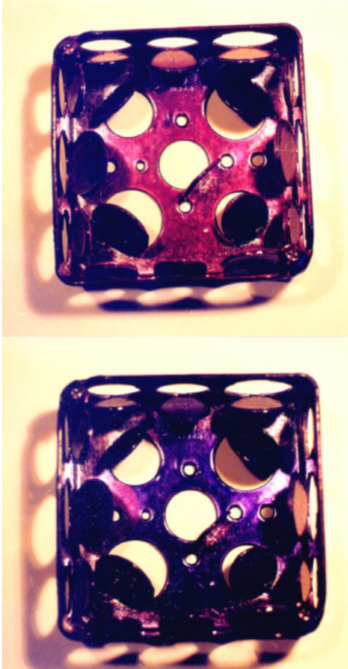
Fig. 7. This test part would present a challenge to position UV lamps. The top photo shows the part prior to UV exposure. The bottom photo reveals UV Distribution on the surface. Note the UV shadows on this part appear as pink areas.
