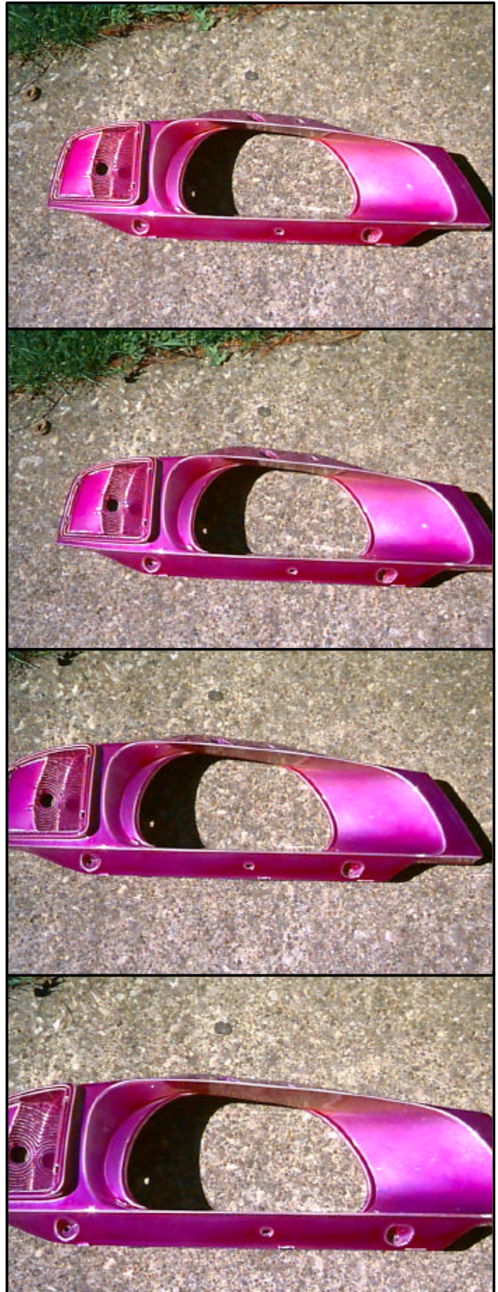
Fig. 3. As the 3DR begins to respond to UV (Top) the part changes color revealing surface variations in UV exposure.
