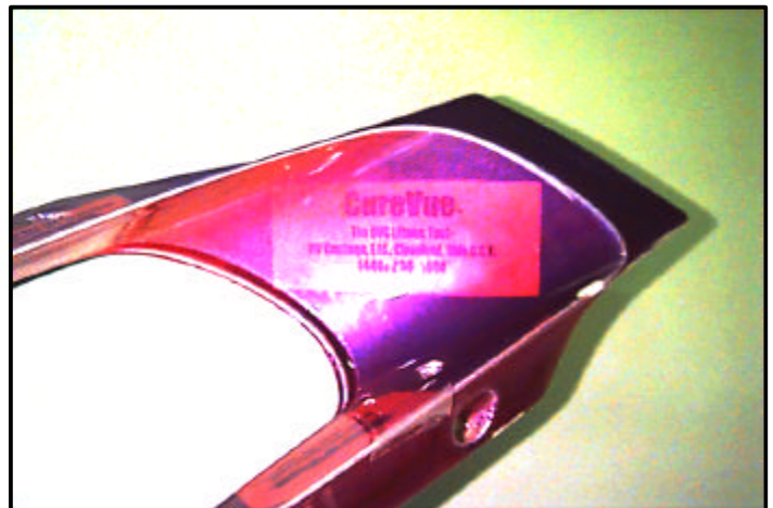
Fig. 2. The same automotive part from Fig. 1. after UV exposure. Note the effect of UV blocking film laid on the part had on the 3DR indicator underneath.
